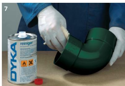
7 Clean the inside of the fitting
