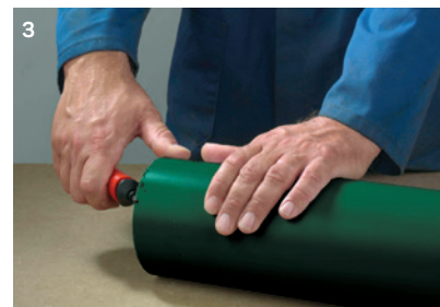
3 Remove the sharp edges on the outside
