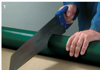
1 Cut the pipe perpendicularly
